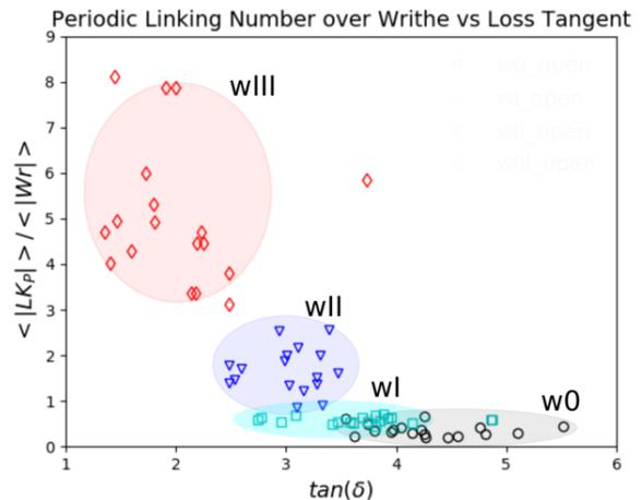
Figure 9. The ratio of the Periodic Linking Number over the Writhe as a function of the loss tangent for open systems at low frequencies. We see that the ratio  $\langle |LK_P| \rangle / \langle |Wr| \rangle$  decreases with the loss tangent. We also find the data can be fit to a relation of the form  $\langle |LK_P| \rangle / \langle |Wr| \rangle \sim (\tan \delta)^{-2.6}$ .
