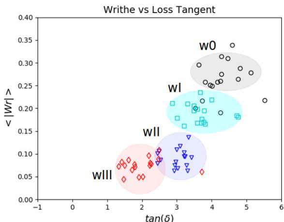
Figure 6. Writhe and Loss Tangent of open chains for small frequencies of oscillation (frequencies corresponding to periods  $T > 6\tau_D$ ). We find a linear behavior of the Writhe as a function of the Loss Tangent. The data points corresponding to the different weaves form clusters. As the topological complexity of the weave decreases both the Writhe and Loss Tangent increase.
