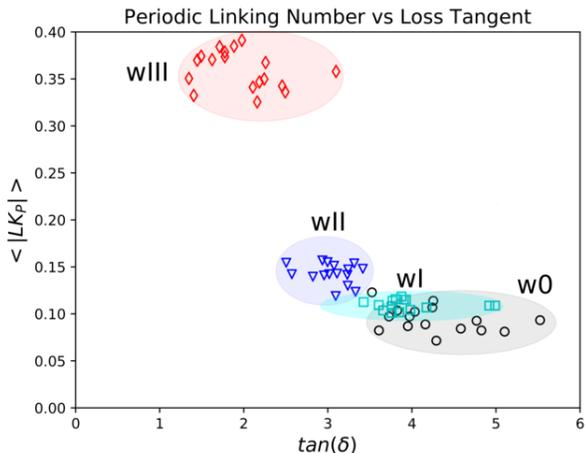
Figure 8. Periodic Linking Number and Loss Tangent of open systems for small frequencies of oscillation (corresponding to periods  $T > 6\tau_D$ ). We find that the responses corresponding to the different weaves form clusters. The Periodic Linking Number increases with weave complexity and decreases with loss tangent.
