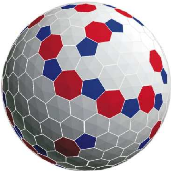
FIG. 5: (Color Online). A Voronoi diagram for the cylindrical phase on a sphere of radius R = 20.0 R_{g0} , with f = 0.8 and \chi N = 25.0 . The sphere consists of 446 microdomains (69 5-fold, 350 6-fold, and 57 7-fold coordinated sites) and exhibits grain boundary scars.
