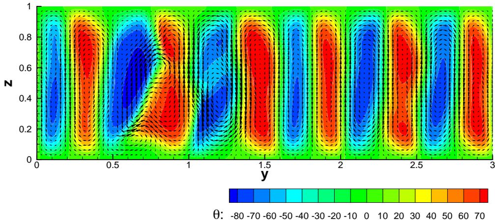
Figure 3: Velocity and director profiles for  $Er = 300$  [ $\tau = 200$  (strain units)]. The vector plot represents the secondary flow components  $v_y$  and  $v_z$ . The overlying contour plot is the angle  $\theta$  between the director and the  $y$ - $z$  plane. The relative magnitudes of  $v_y$  and  $v_z$ , with respect to the shear component  $v_x$  are  $O(10^{-2})$ .
