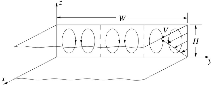
Figure 1: Schematic of the two-dimensional shear flow domain. The flow field is bounded along the spanwise direction by parallel plates separated a distance  $H$  and along the wall-normal direction by periodic boundaries separated a distance  $W$ .  $V$  is the relative velocity between the two plates.
