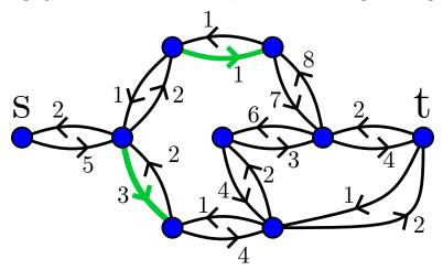
These two edges form a "bottleneck" for our flow, as all paths from the source s to the sink t must go through one of these two edges. However, the maximum capacity of these two edges is 4; therefore, it would seem impossible for any flow to pump more than 4 units out of the source!
