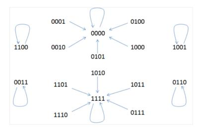
As we can see from this phase space, there are 6 fixed points: 1100, 0011, 0000, 1111, 1001, and 0110. In order to figure out how many fixed points there are, we first had to generate the phase space. This requires a large amount of work, that increases by a power of 2 for a step from  $\operatorname{Circ}_n$  to  $\operatorname{Circ}_{n+1}$ . If we want to know how many fixed points a  $\operatorname{Circ}_n$  graph has without having to draw the phase space, we need some other method.
