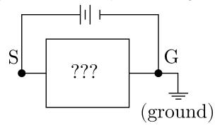
In this sense, we can simply "abstract" the rest of our circuit as some particularly large and bulky resistor, with effective resistance (which we denote  $R_{\text{eff}}$ ) given by Ohm's law:
