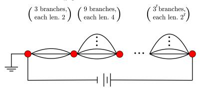
By applying our known results about resistors in series and parallel, we can see that the total resistance between any two nodes n - 1, n in the above circuit is
