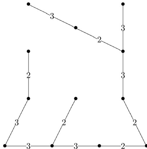
The process is complete since the addition of any other edge would create a cycle. Alternatively, we could note that the original graph had 12 vertices and we have already selected  $11 = 12 - 1$  edges.
