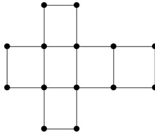
**Solution:** An Eulerian circuit is a closed trail that contains each edge of a graph. We saw in class that a connected graph is Eulerian if, and only if, each vertex has even degree. The vertices indicated below both have degree 3, which is odd. Hence, the graph cannot be Eulerian.
