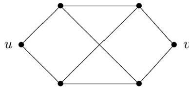
**Solution:** First we subdivide the resistors to get a graphical representation where all the edges represent a resistance of one ohm. Then we label the vertices.
