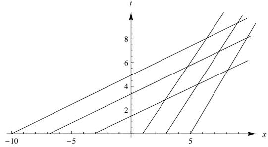
Figure 3.4: Characteristic lines illustrating shock wave formation.
