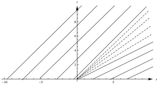
Figure 3.3: Characteristic lines illustrating rarefaction.
