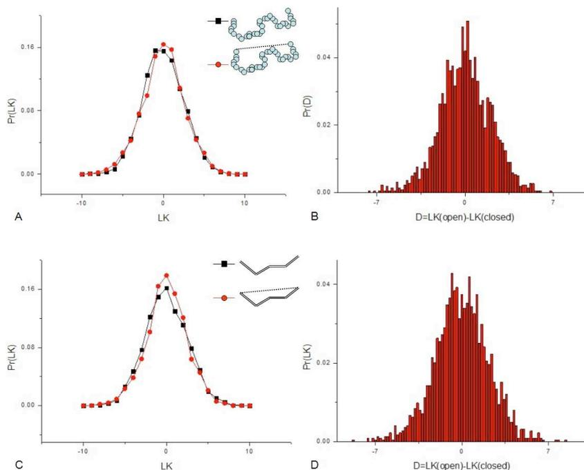
Fig. 4. Figure A shows the normalized probability distribution of  $LK$  for the original chains before and after end-to-end closure and Figure B the probability distribution of the corresponding differences. Figure C shows the normalized probability distribution of  $LK$  for the reduced chains before and after end-to-end closure and Figure D shows the corresponding differences
